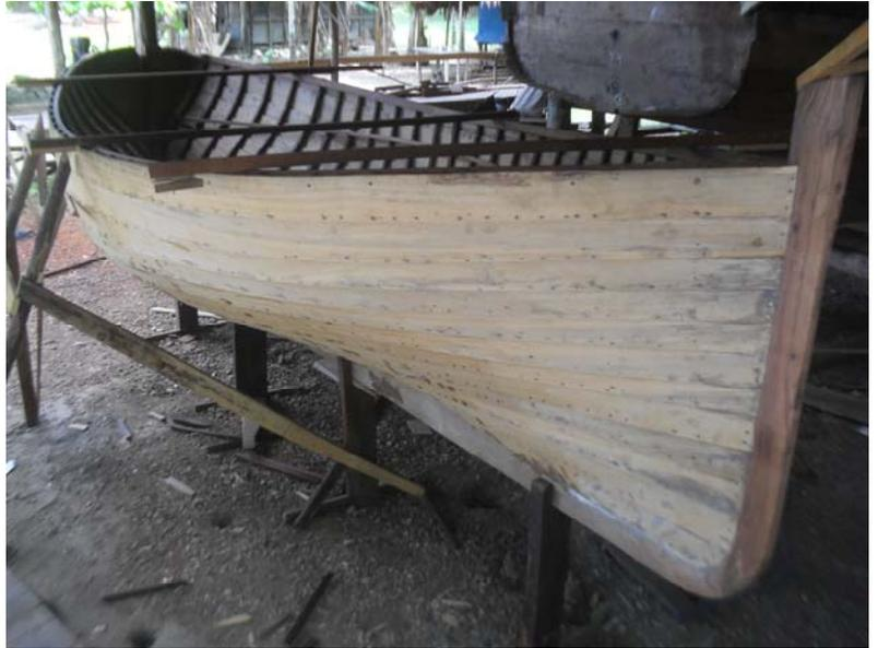
together). Rosewood (*pterocarpus indicus*) has been cut for the thwarts and seats but the *bush calophyllum* for the spars is still being straightened under tension. The last few days of work before the break for Christmas will probably see the seating done and a start made on the rudder.
