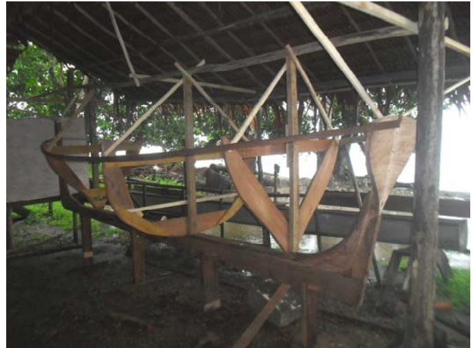
Lema set up and ready for planking up
